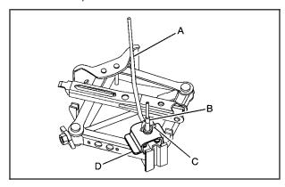
3. Place the jack over the bolt (B) on the floor, making sure it contacts the bolt as shown.
